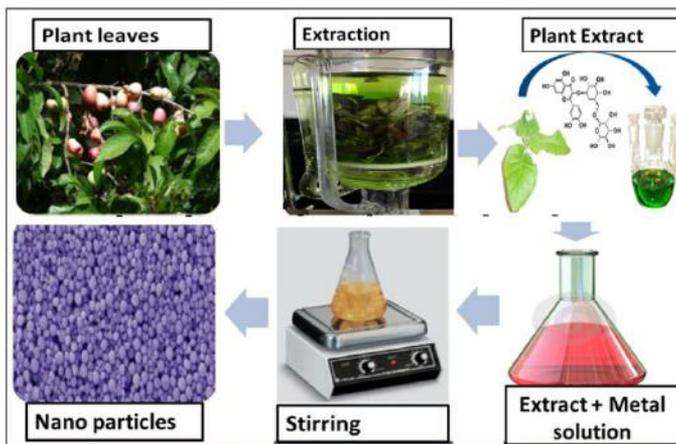
**Fig 2:** A schematic diagram of green synthesis of metal nanoparticles from plant extracts
