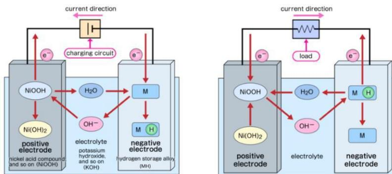
**Fig 7:** Charging and discharging state of NiMH batteries <sup>[24]</sup>.
