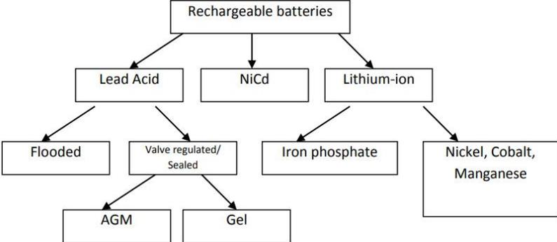
**Fig 3:** Classification of rechargeable batteries used in EVs [16]
