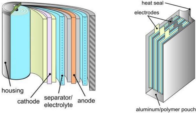
**Fig 11:** Lithium-ion cell construction <sup>[37]</sup>
