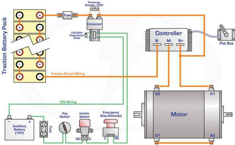
**Fig 2:** Schematic diagram of an electric vehicle wiring from battery <sup>[14]</sup>
