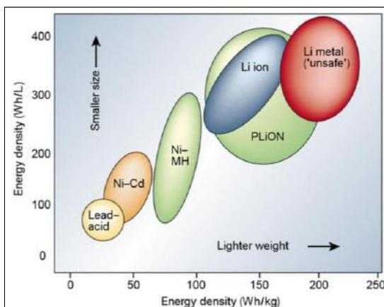
**Fig 12:** Energy density profile of batteries <sup>[38]</sup>
