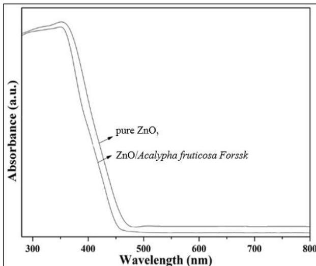
**Fig 2:** Diffuse reflectance spectra of pure ZnO, ZnO/*Acalypha fruticosa Forssk* and ZnO/*Acalypha fruticosa Forssk*/curcumin nanoparticle
