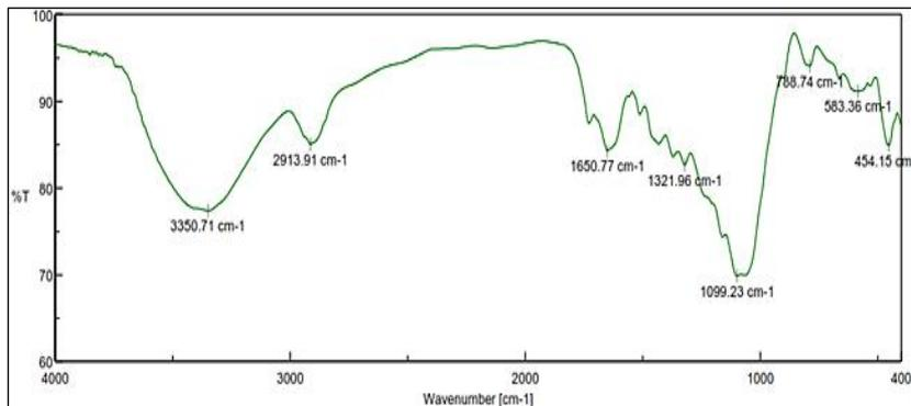
**Fig 1:** FT-IR spectrum of ZnO/*Acalypha fruticosa Forssk* nanoparticles.
