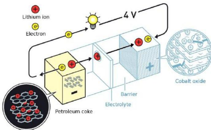
**Modern commercial Li-ion battery using Coke based anode and  $\text{Li}_x\text{CoO}_2$  cathode**
