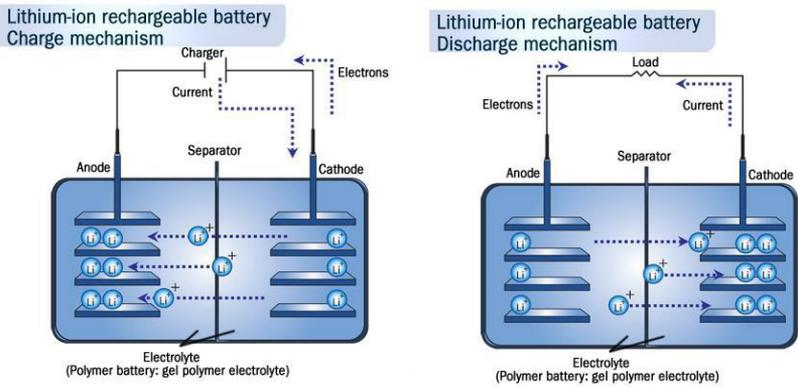
**Fig 9:** Intercalation mechanism during charging and discharging of Lithium-ion battery <sup>[35]</sup>
