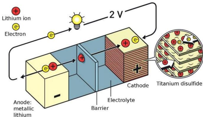
**Lithium-based battery using  $\text{Li}_x\text{TiS}_2$  as the cathode.**
