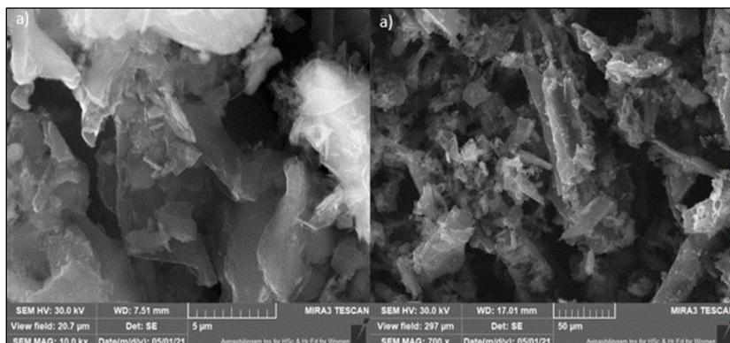
**Fig 3:** SEM images of Pure a) ZnO and b) ZnO/*Acalypha fruticosa* Forssk nanoparticles
