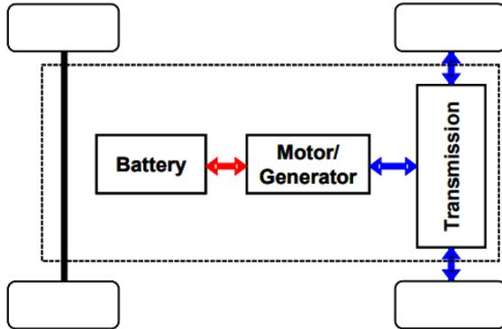
**Fig 1:** Schematic of a battery electric vehicle (BEV) powertrain <sup>[11]</sup>
