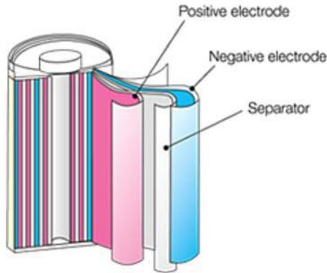
**Fig 8:** Schematic diagram of cylindrical NiMH battery construction <sup>[28]</sup>.
