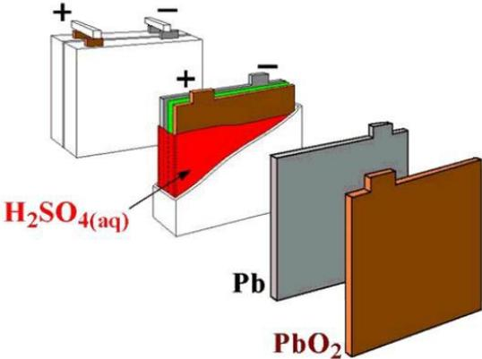
**Fig 5:** Schematic diagram of Lead-acid battery [21]
